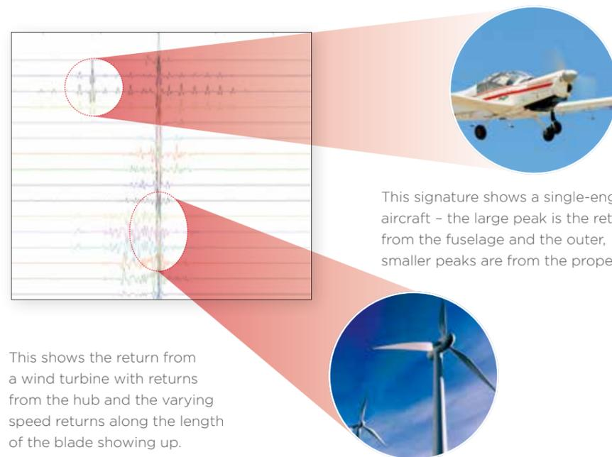
This signature shows a single-engined aircraft – the large peak is the return from the fuselage and the outer, smaller peaks are from the propeller.
