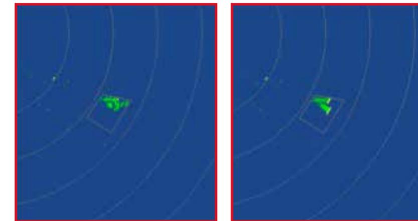
Actual screenshot showing a PSR display with and without the Holographic Radar™ infill. The left-hand shot shows the display that the controller would see, with the aircraft ‘lost’ within the turbine clutter. The right-hand shot shows the turbine removed, and a clear display of the aircraft tracks from the Holographic Radar™.
